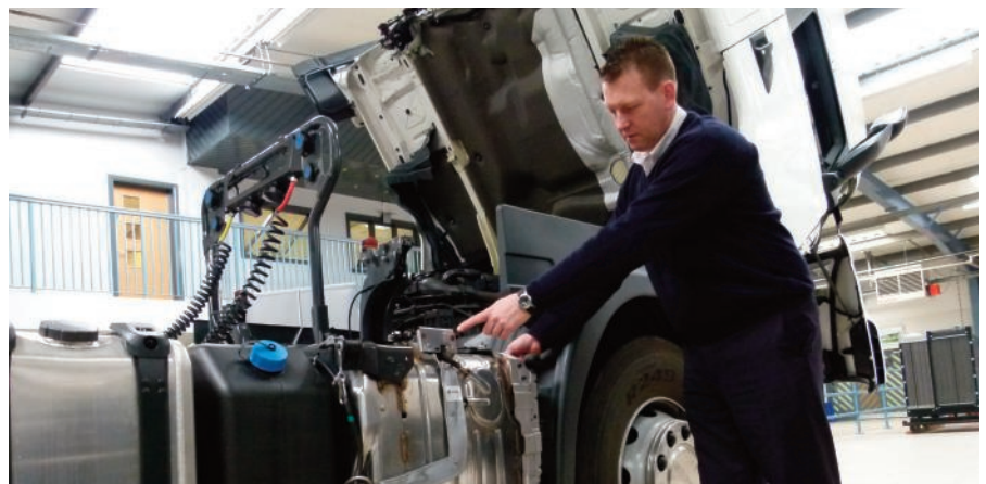
Euro 6 trucks' after-treatment packages have multiple sensors that monitor system health
