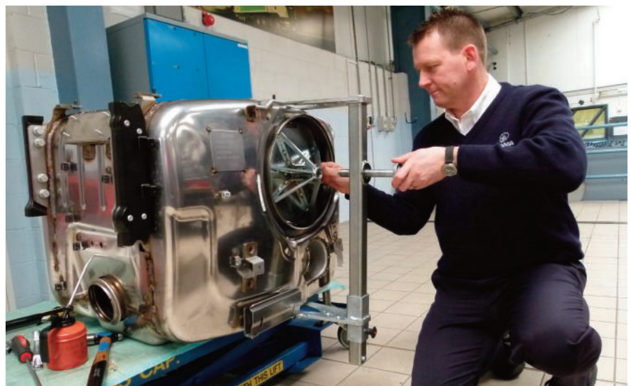
Scania's Keith Gallon prepares to extract a DPF assembly
